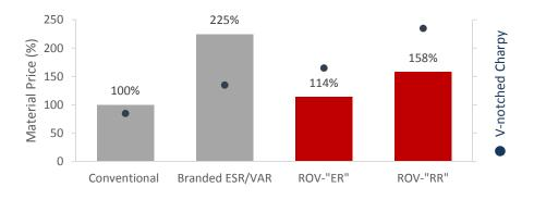
For the Rovalma grades, V-notched Charpy values have been obtained in samples taken from the center of a 850 x 445 mm bar, hardened at 1020 °C for 30 min., quenched in air and tempered twice. Final hardness was 44-46 HRc.
